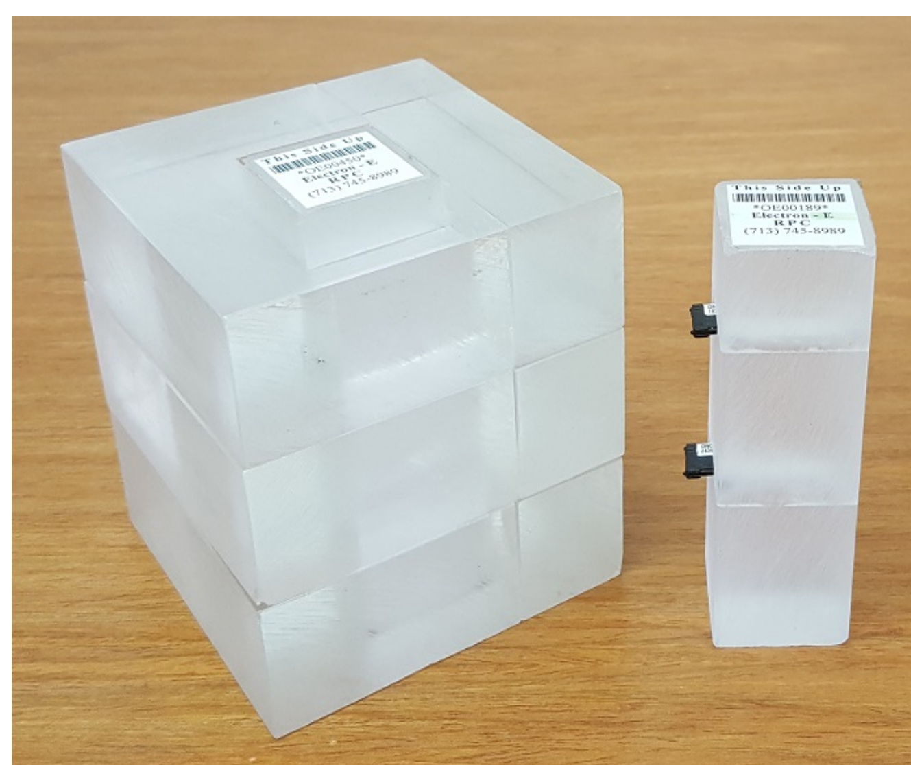
Figure 1: Electron beam block and special insert for 16 MeV electron beam with OSLD at both levels
